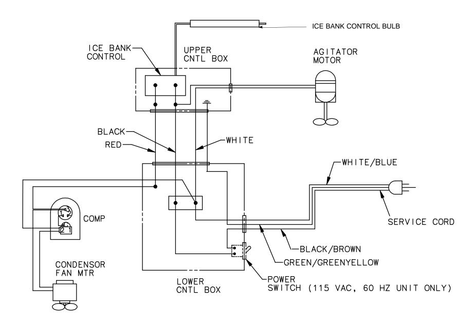
**FIGURE 4. UNIT WIRING DIAGRAM**
